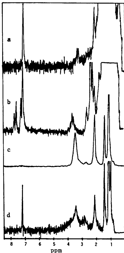
Fig. 2. ^1\text{H-NMR} spectra of: \alpha,\omega -di-(hydroxy)polyisobutylene ( \bar{M}_n = 4,780 ) (a); \alpha,\omega -di(tosyl)polyisobutylene ( \bar{M}_n = 6,100 ) (b); poly( N -acetyleneimine- b -isobutylene- b -acetyleneimine) (Sample 2, Table 2) (c); poly(ethyleneimine- b -isobutylene- b -ethyleneimine) (d)
